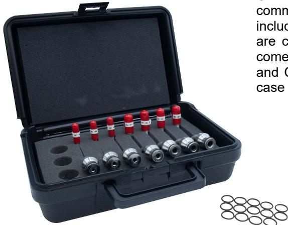
Our Stainless Steel Nozzle Sets include a selection of the most commonly used sizes. Each set contains seven nozzles which include sizes 4, 5, 6, 7, 8, 9, 10. Our Stainless Steel Nozzle Sets are constructed of a seamless Stainless Steel alloy. All nozzles come with a standard 5/8 inch OD shank with an integrated ferrule and O-ring to minimize leaks. Packaged in a foam-lined carrying case for protection.
