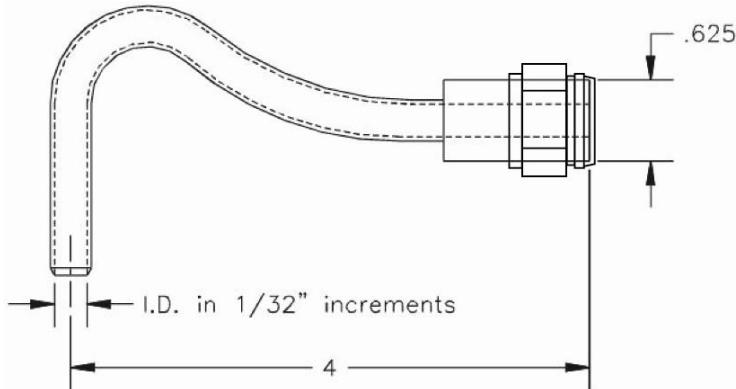
Our Inconel Nozzle Sets include a selection of the most commonly used sizes. Each set contains seven nozzles which include sizes 4, 5, 6, 7, 8, 9, 10. All nozzles come with a standard 5/8 inch OD shank with an integrated ferrule and O-ring to minimize leaks. Packaged in a foam-lined carrying case for protection.
