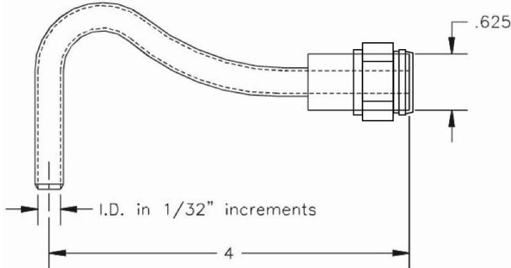
Our Inconel Nozzle Sets include a selection of the most commonly used sizes. Each set contains seven nozzles which include sizes 4, 6, 8, 10, 12, 14, 16. All nozzles come with a standard 5/8 inch OD shank with an integrated ferrule and O-ring to minimize leaks. Packaged in a foam-lined carrying case for protection.
