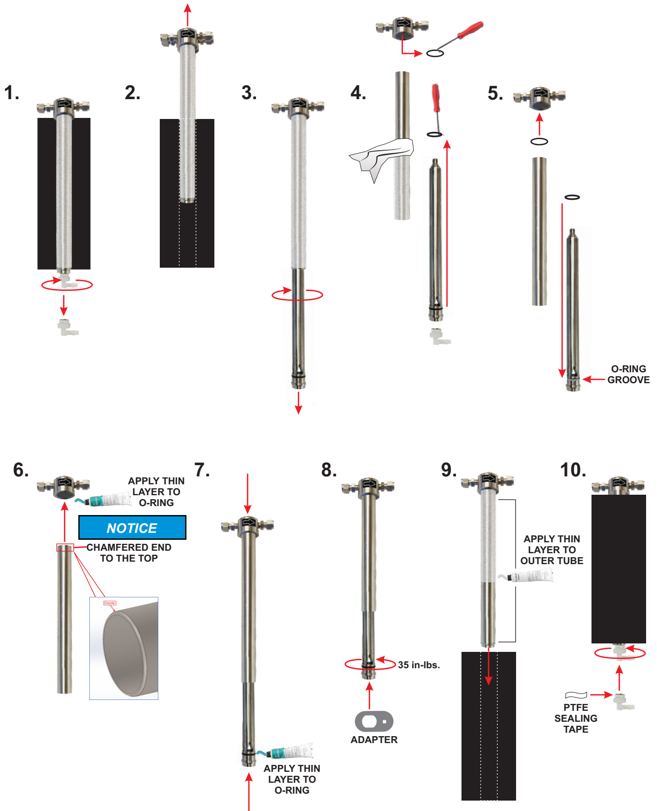
Fig. 9 SC-1612 DISASSEMBLY AND REASSEMBLY
