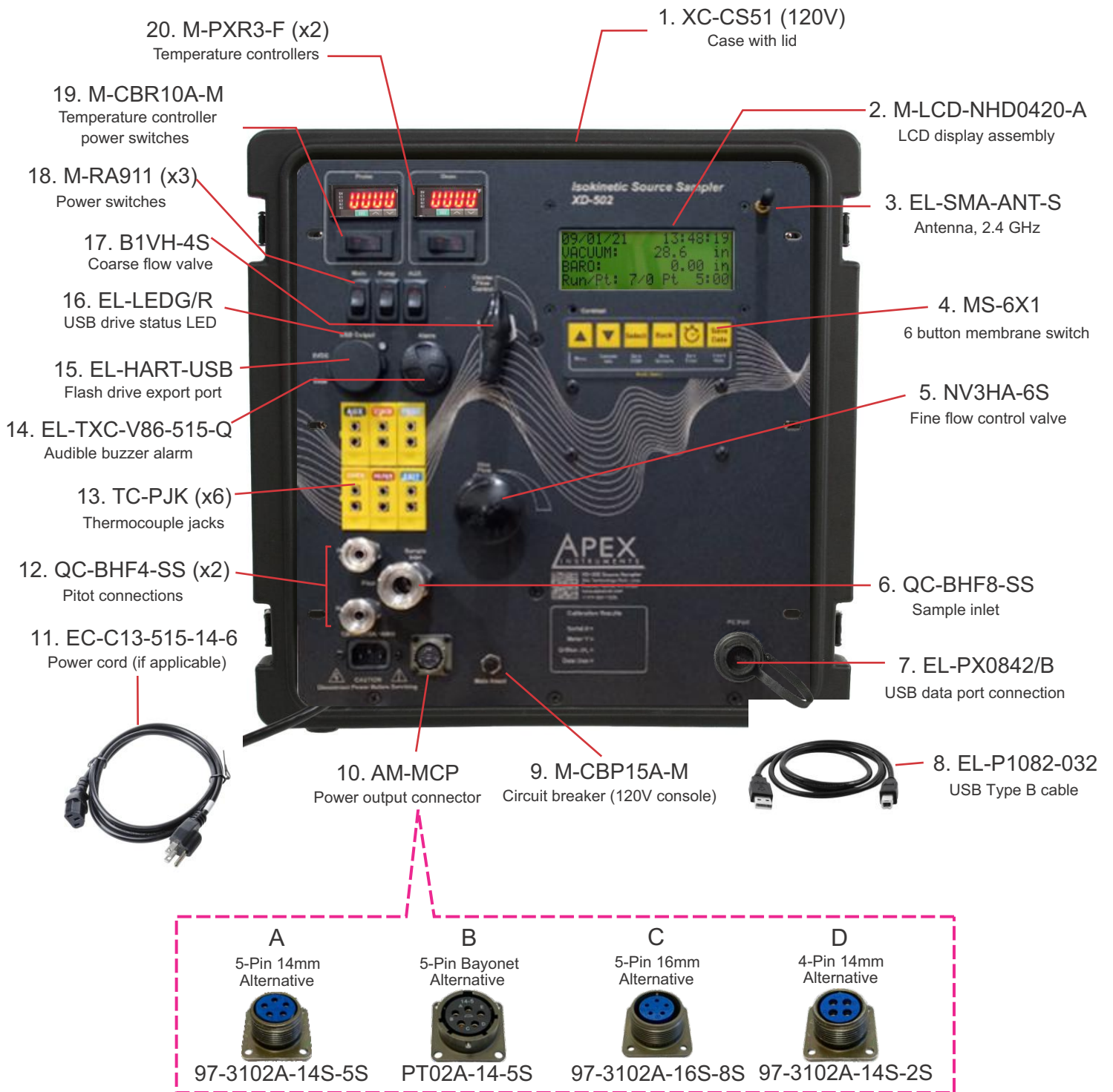
Fig. 23 Parts List (Front Panel) - Standard version shown, depiction of options may differ
