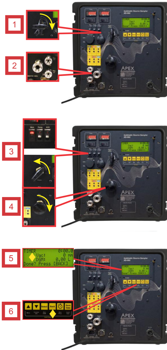
Fig. 5 Front-Side Leak Check
