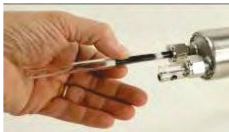
Inserting the traps into the probe
