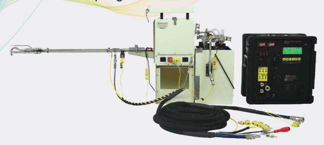
Using the Method 5 Sampling System, particulate matter is withdrawn isokinetically from the source and collected on a glass fiber filter maintained at a temperature of 120 ±14 °C (248 ±25 °F) or such other temperature as specified by an applicable subpart of the standards or approved by the administrator for a particular application. The PM mass, which includes any material that condenses at or above the filtration temperature, is determined gravimetrically after the removal of uncombined water.
