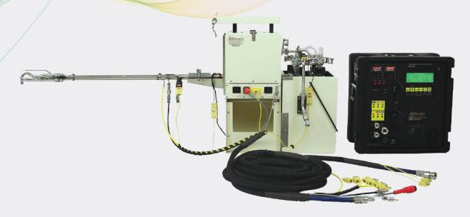
The Apex Instruments Method 26A sampling train is used for the determination of hydrogen halide and halogen emissions. Method 26A is the isokinetic alternative to Method 26. This method is particularly suited for sampling sources controlled by wet scrubbers emitting acid droplets. The method requires a Method 5 sampling train with the use of additional impingers, reagents, and PTFE-coated glass fiber filter media.
