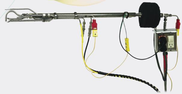
The compact Method 5 kit does not require a separate heated filter compartment and utilizes a flexible sample line and a split umbilical cord with a power adapter to allow sampling in space-limited areas.
